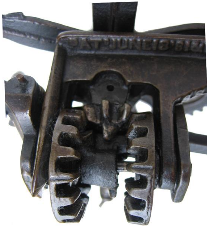
Fig. 4 Differential Gearing Mechanism of the Double Action Apple Parer
