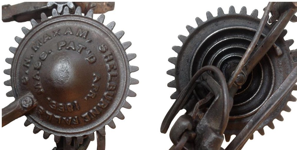
G. H. Hubbard's use of the Scroll Wheel on the 2-Arm Maxam
